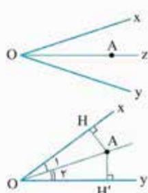
$$\begin{array}{c|c} \text{فرض} & \hat{O}_1 = \hat{O}_2, AH \perp Ox, AH \perp Oy \\ \hline \text{حكم} & AH = AH' \end{array}$$
